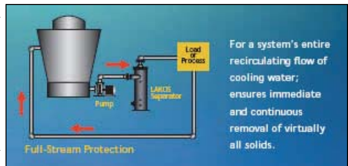
Picture #4 - Full-Flow Filtration
